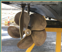
VAR Rudder installed for sea trials
